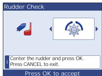
2. Press OK to display the **Rudder Check** (port) page.
