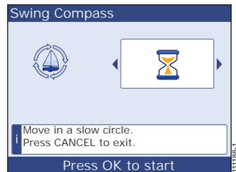
2. When calibration is complete, a message will be displayed showing the detected deviation. If deviation is more than 5 degrees:
