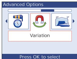
2. Press **OK** to display the **Variation** setup box. This has two adjust boxes, an upper box which shows the variation mode, and a lower box that shows the variation value.
