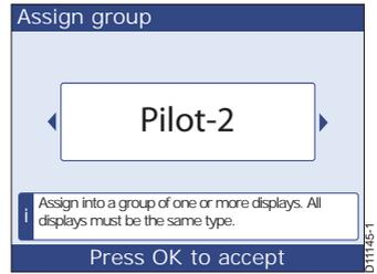
7. Press OK to save the group assignment and display the **Assign order in group** page. Each display in a group has a discrete number, and these numbers determine the order in which displays are selected within the group during normal operation, when the Select Display button is used.
