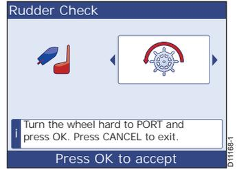
4. Press OK, to display the **Rudder Check** (starboard) page.
