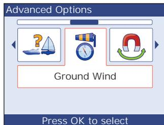
4. Press **OK** to display the **Ground Wind** setup box.
