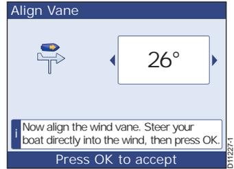
If there is any inaccuracy after you have completed the wind vane alignment, then:
